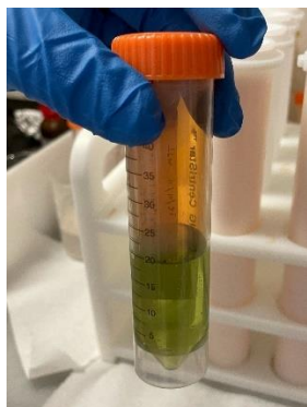
Figure 3. Image of microwave digested LLTZO in H_2SO_4:HNO_3:H_2O_2 showing orange gas evolved.
